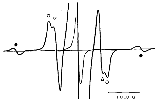
Figure 3. ESR spectrum of the monoradical (C 6 Cl 5 ) 2 C•-C 6 Cl 4 -COOCH 2 -CH 2 OH in CCl 4 at room temperature. 13 C line pairs: \alpha , ●; bridgehead, ○; ortho, ▽.
